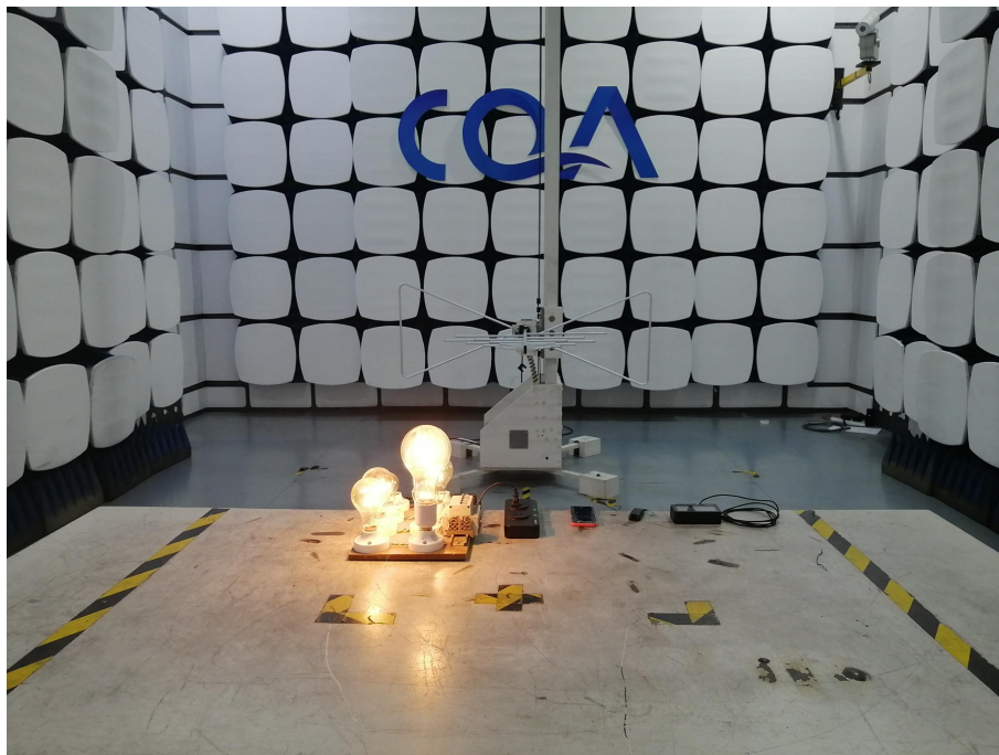
Radiated emission Test Setup (30MHz~1GHz)
