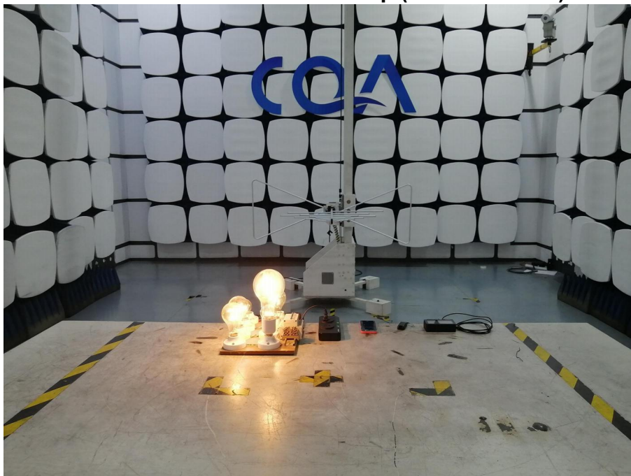
Radiated emission Test Setup (30MHz~1GHz)
