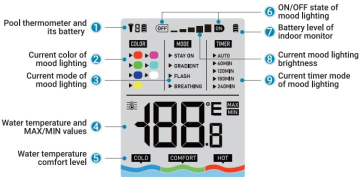
**1 Pool thermometer and its battery level:** It shows the current channel and its battery level. When the channel is switched to 0, all bound channels will be displayed in turn every 2 seconds. When the icon flashes, it means that the battery of the corresponding pool thermometer is too low.
