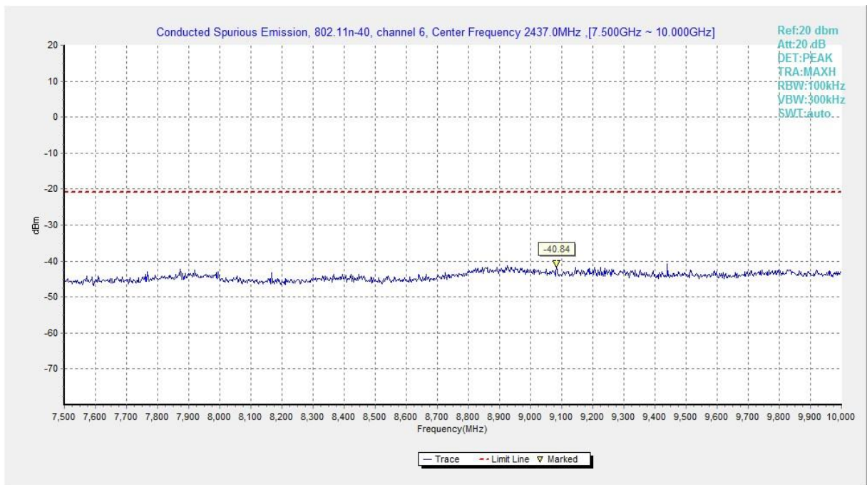
Fig.B.6.1.85 Transmitter Spurious Emission - Conducted (802.11n-HT40, Ch6, 7.5 GHz-10 GHz)
