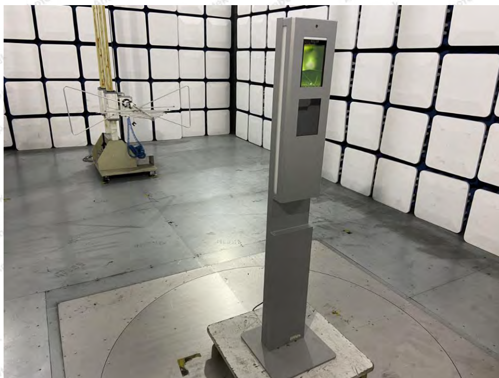
Photo of Radiation Emission Test
