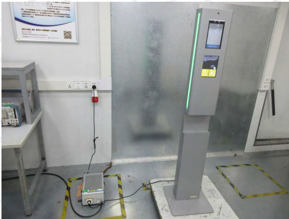
Photo of Conducted Emission Measurement
