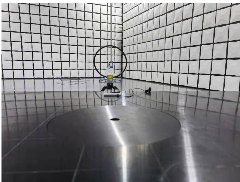
Conducted Emissions Test Setup (with charger)
