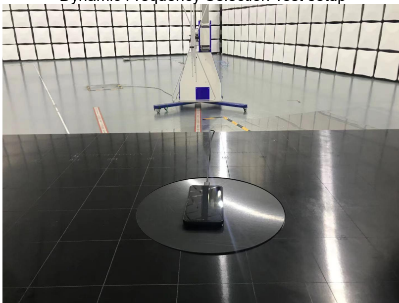
Dynamic Frequency Selection Test setup
