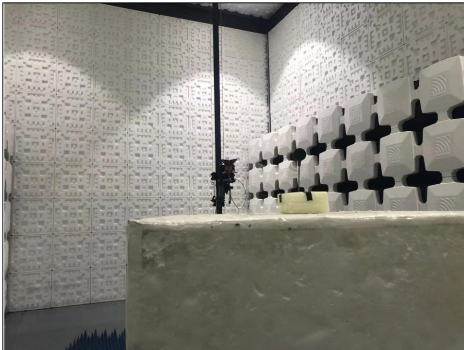
Radiated emission above 1G
