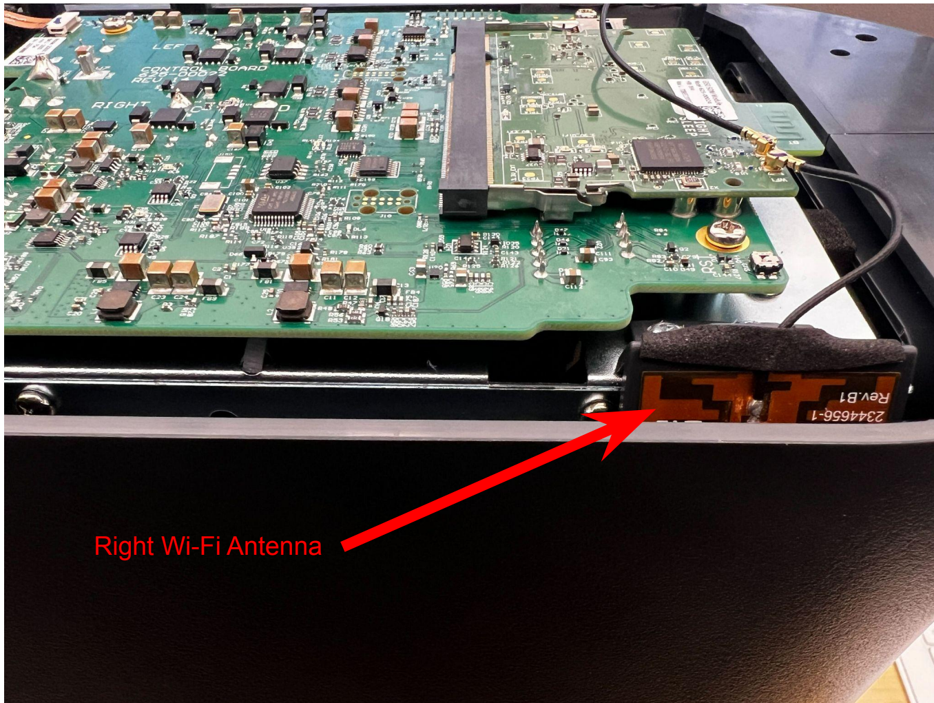
Right Wi-Fi Antenna
