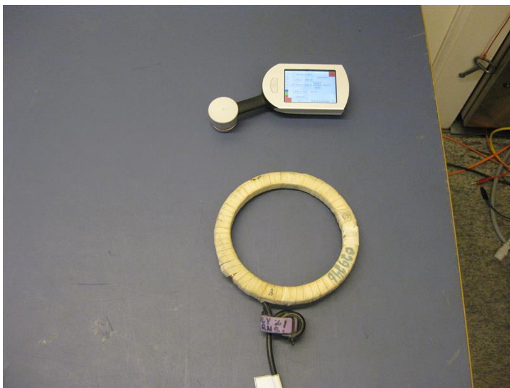
Photo 4.5.2 Test set-up regarding measurement of 20 dB bandwidth
