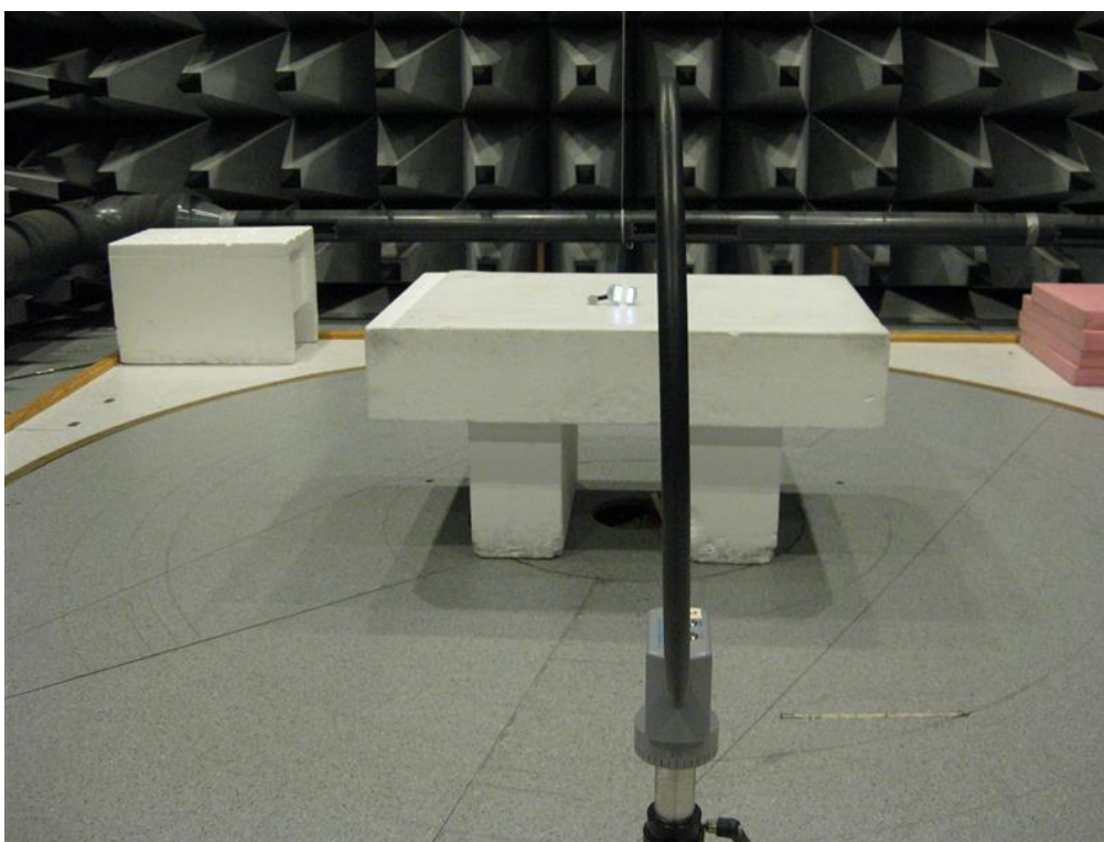
Photo 4.1.2 Test set-up regarding measurement of radiated emission (below 30 MHz).
