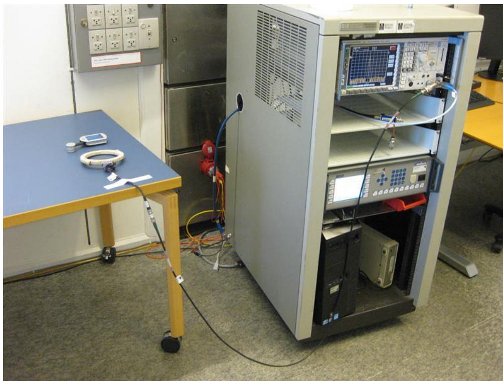
Photo 4.5.1 Test set-up regarding measurement of 20 dB bandwidth
