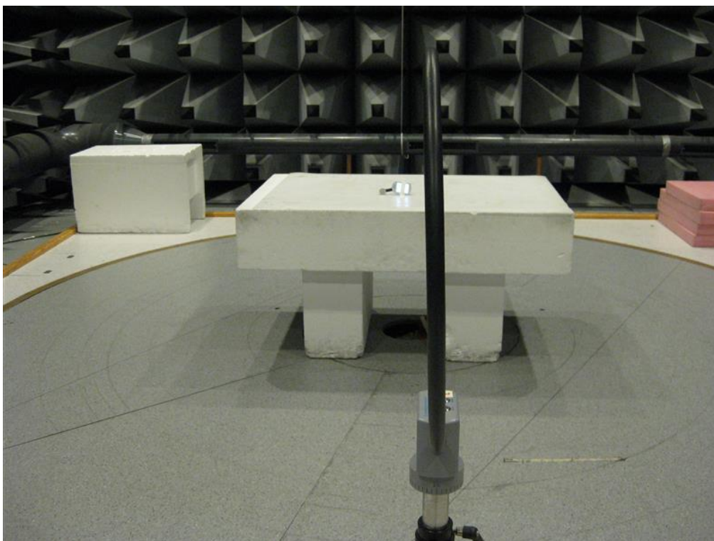
Photo 4.1.2 Test set-up regarding measurement of radiated emission (below 30 MHz).
