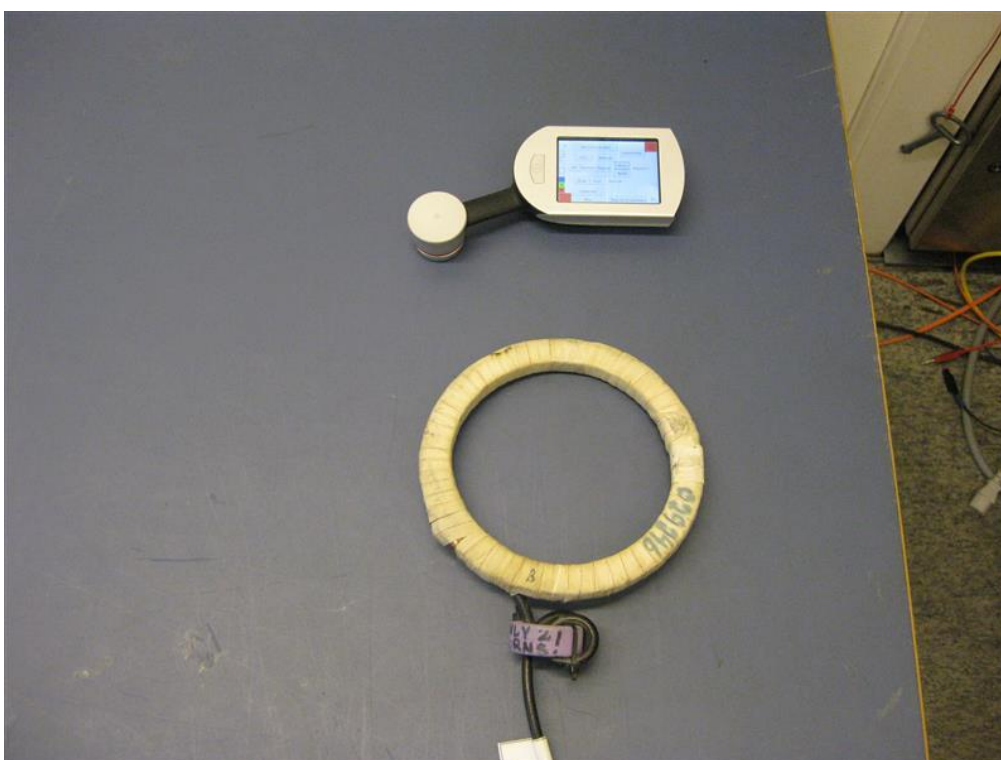
Photo 4.5.2 Test set-up regarding measurement of 20 dB bandwidth
