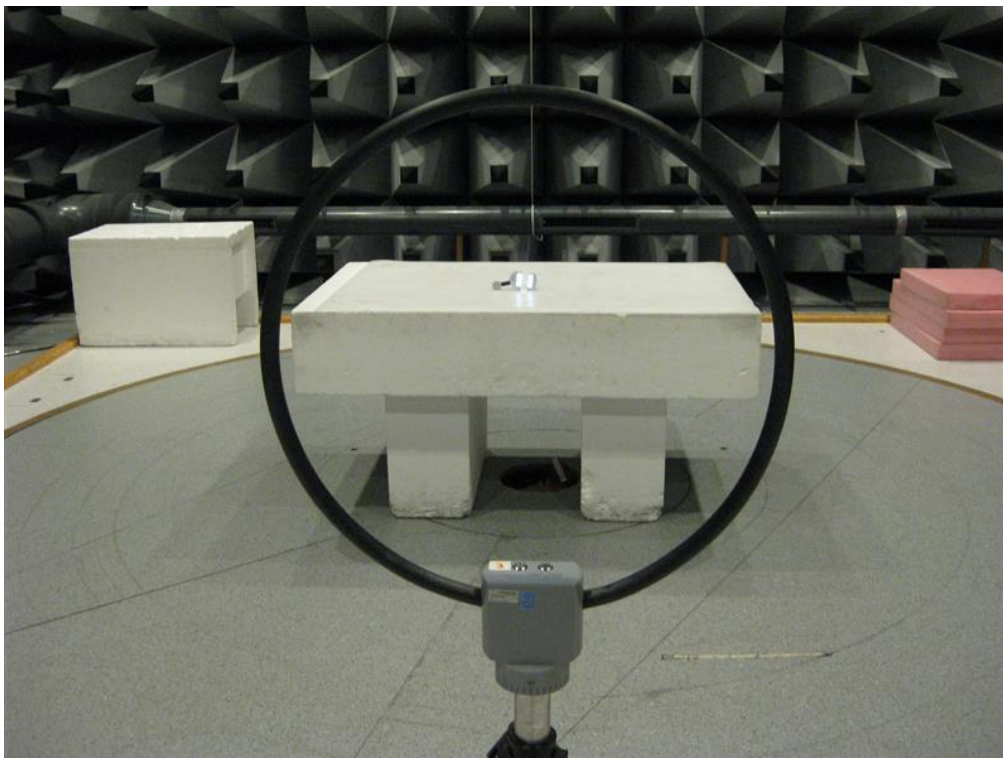
Photo 4.1.1 Test set-up regarding measurement of radiated emission (below 30 MHz).
