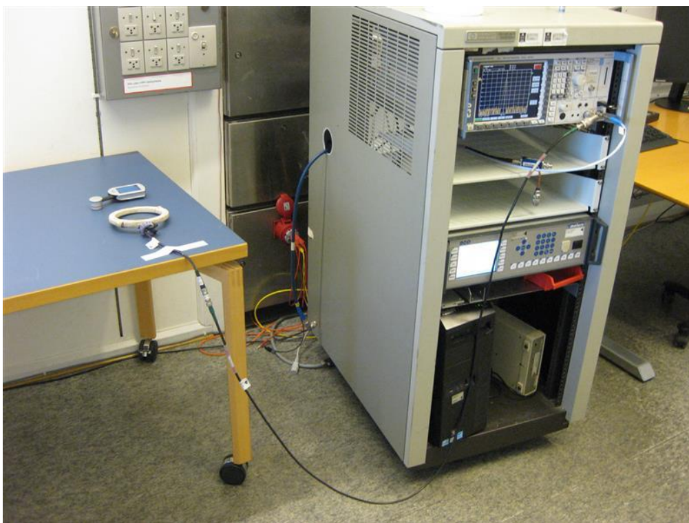
Photo 4.5.1 Test set-up regarding measurement of 20 dB bandwidth
