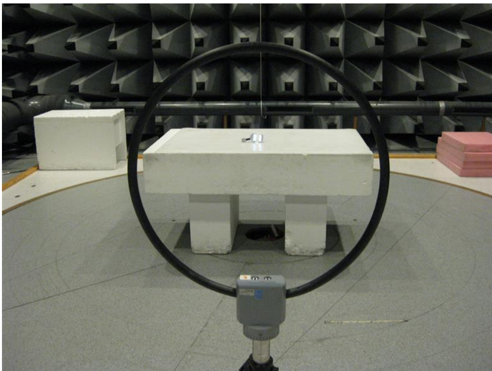
Photo 4.6.1 Test set-up regarding measurement of radiated band edge compliance
