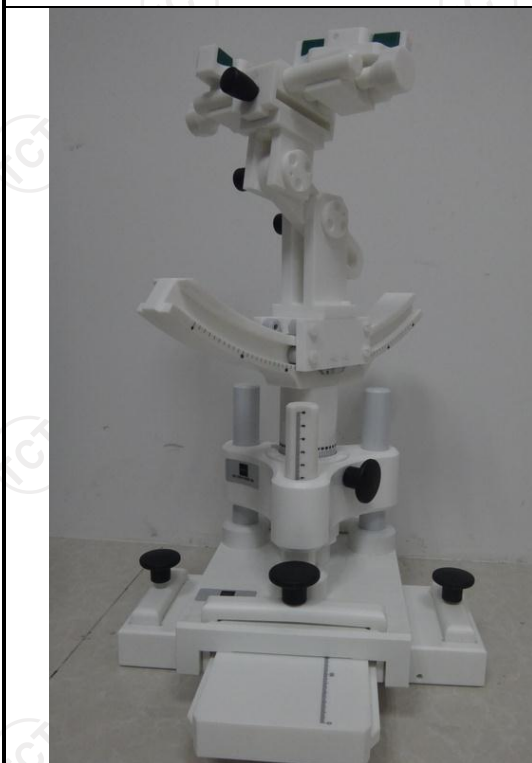
COMOSAR Mobile phone positioning system
