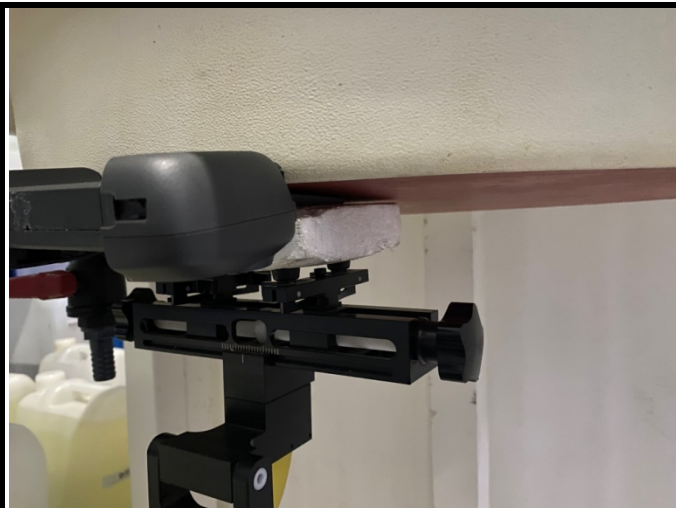
Rear Face of EUT with 0 cm Gap
