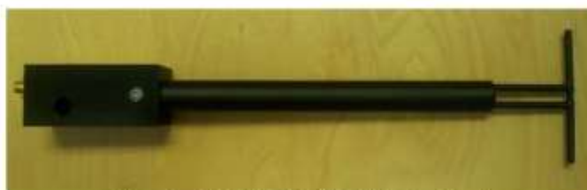
Figure 1 – MVG COMOSAR Validation Dipole
