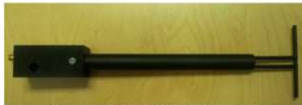
Figure 1 – MVG COMOSAR Validation Dipole
