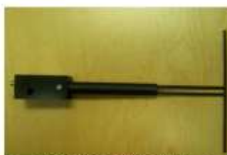
Figure 1 – MVG COMOSAR Validation Dipole
