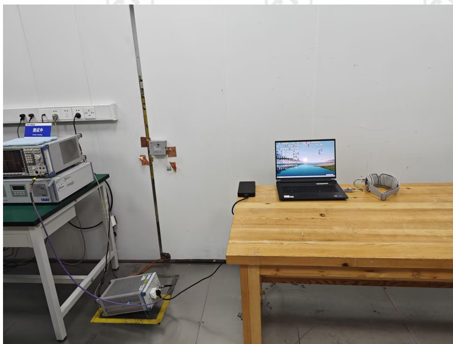
Conducted Emissions Test Setup
