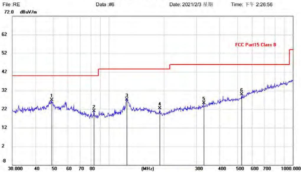
Site Limit: FCC Part15 Class B EUT: True Wireless Earbuds M/N: T7 Mode: TX mode Note:
