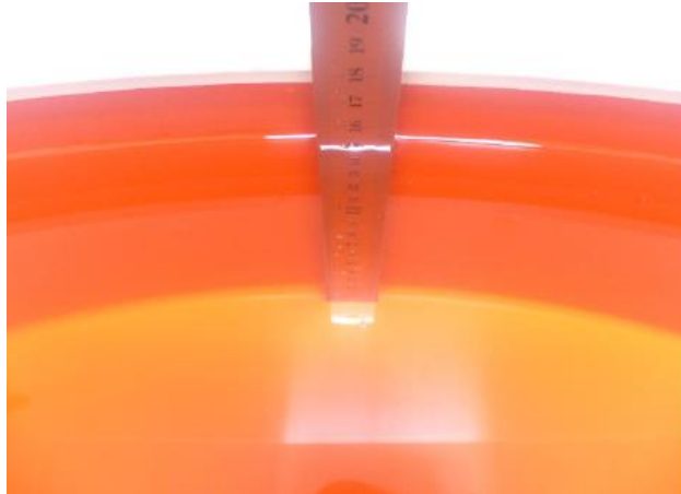
Photo 1: Tissue Simulant Liquid for Head 450MHz
