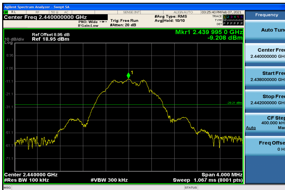
RF Conducted Spurious Emissions_BLE_2440
