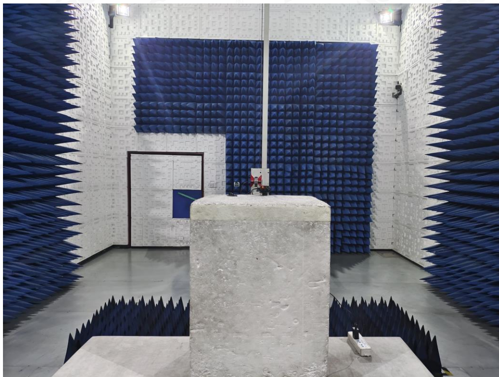
RADIATED EMISSION ABOVE 1G TEST SETUP
