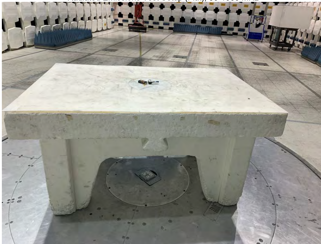
Radiated Emissions Test Setup (Flat), 30-1000 MHz
