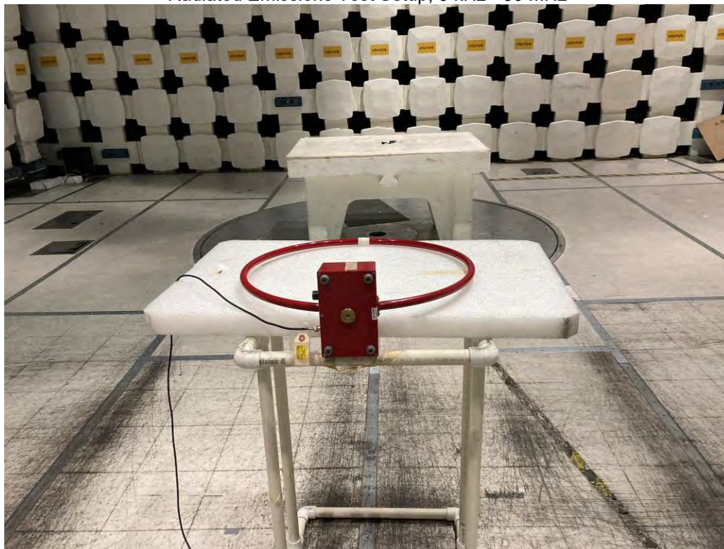
Radiated Emissions Test Setup, 9 kHz - 30 MHz
