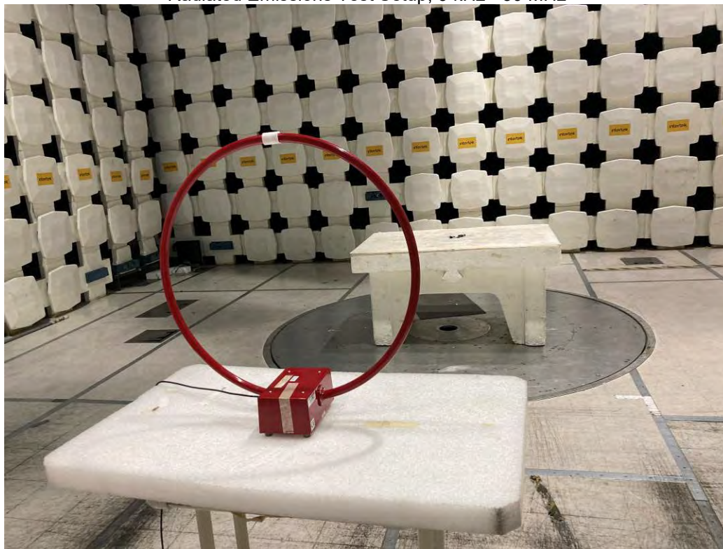
Radiated Emissions Test Setup, 9 kHz - 30 MHz
