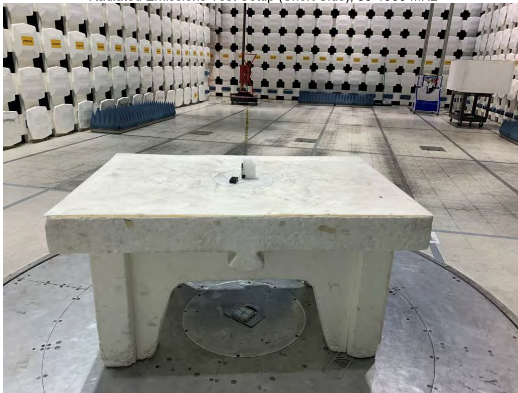
Radiated Emissions Test Setup (Short Side), 30-1000 MHz
