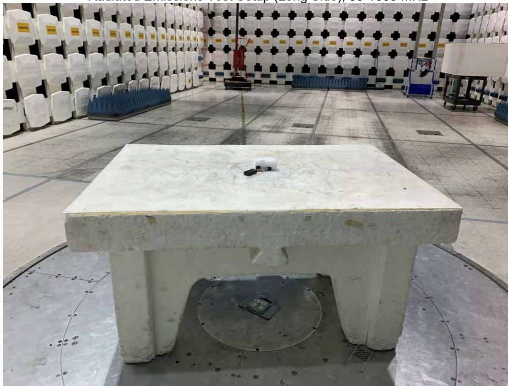
Radiated Emissions Test Setup (Long Side), 30-1000 MHz
