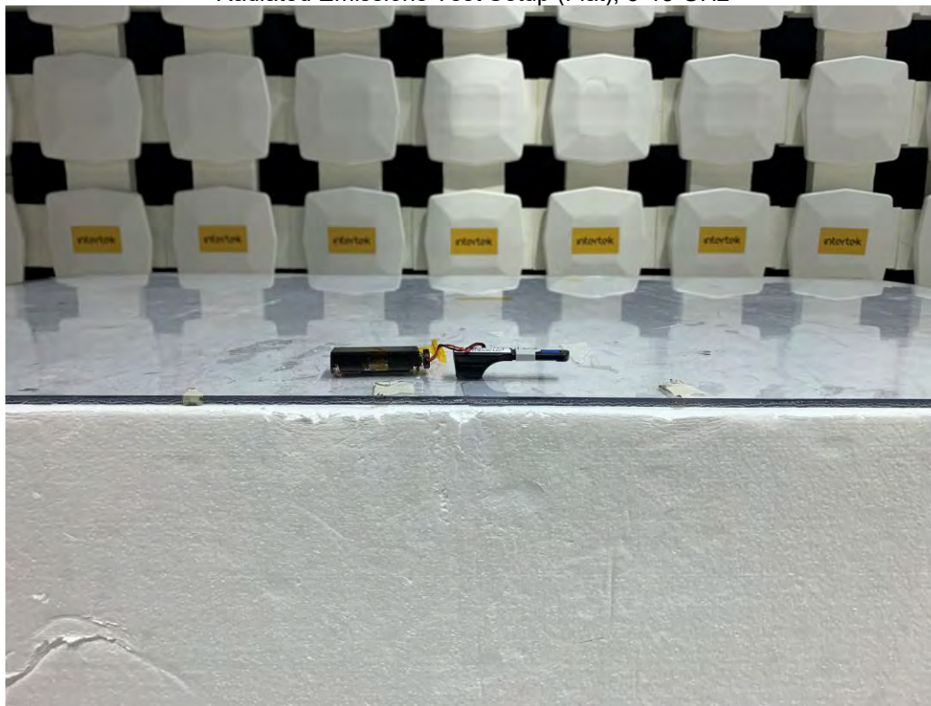
Radiated Emissions Test Setup (Flat), 3-18 GHz
