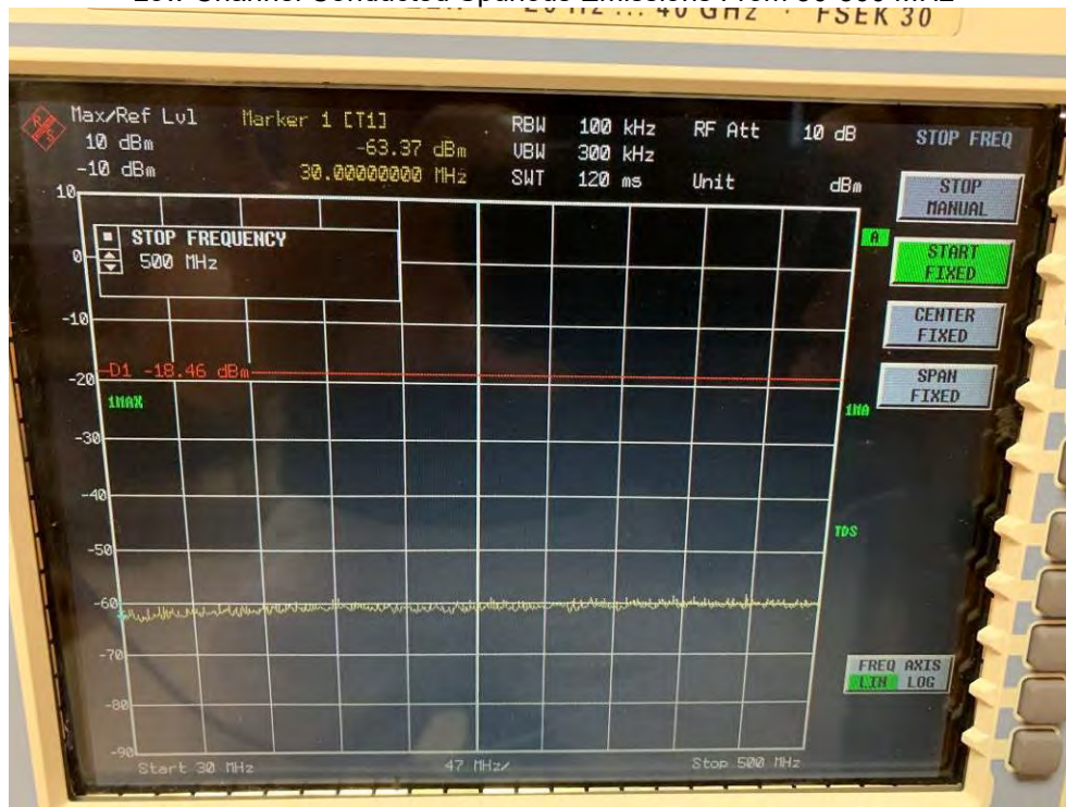
Low Channel Conducted Spurious Emissions From 30-500 MHz
