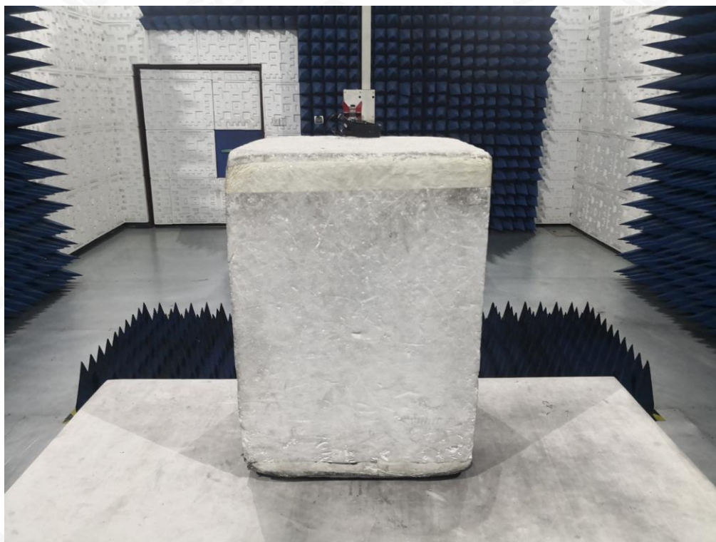
FCC RADIATED EMISSION TEST SETUP ABOVE 1GHZ
