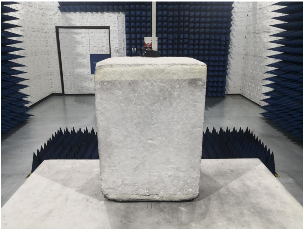
FCC RADIATED EMISSION TEST SETUP ABOVE 1GHZ
