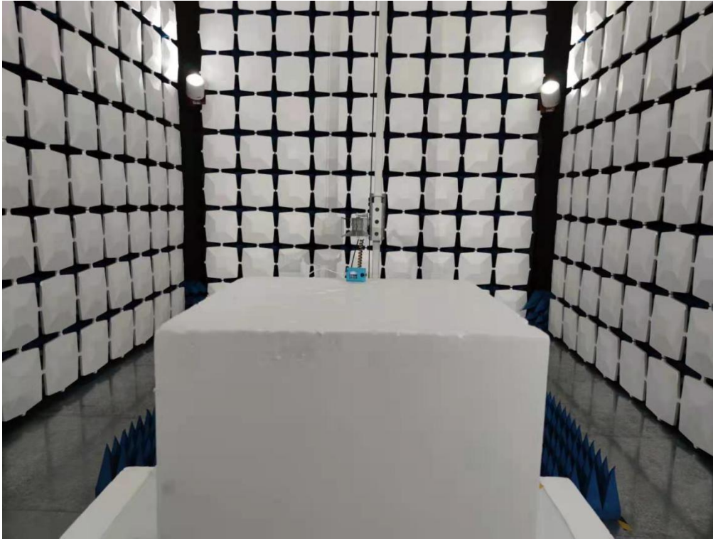
Above 1GHz for radiated emission test setup
