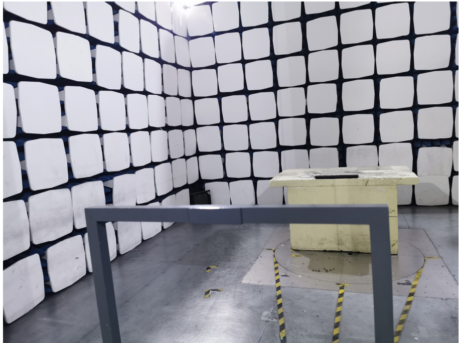
Radiation Emission Test Setup (Below 30MHz)
