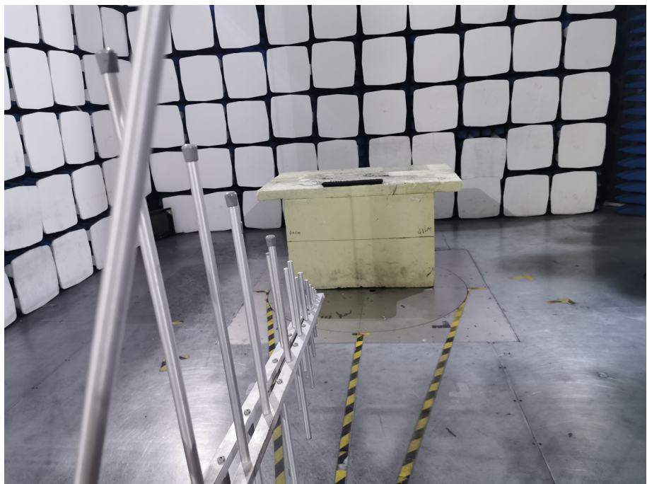
Radiation Emission Test Setup (30MHz to 1GHz)
