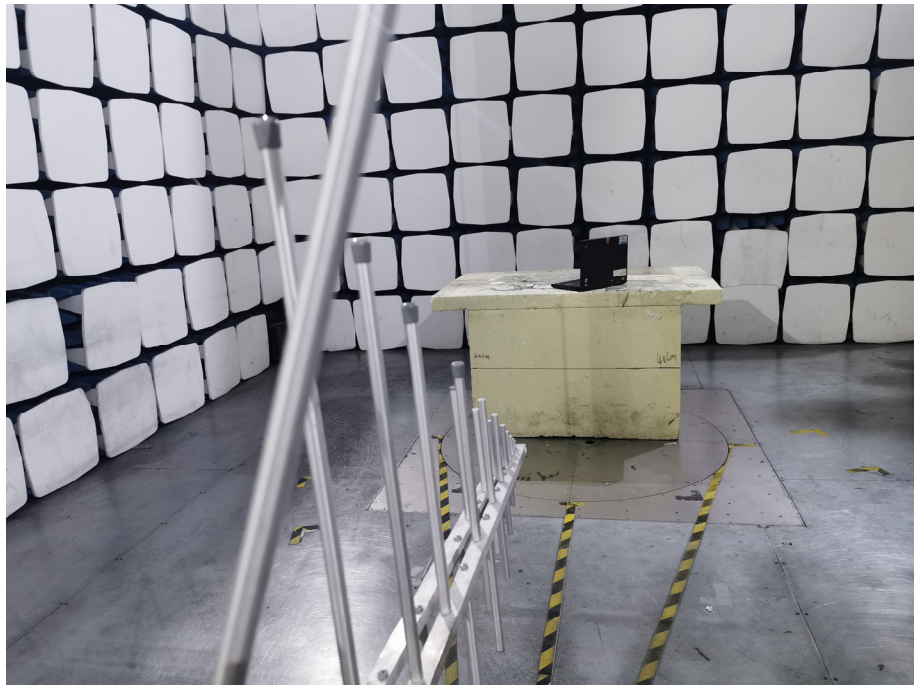
Radiation Emission Test Setup (30MHz to 1GHz)
