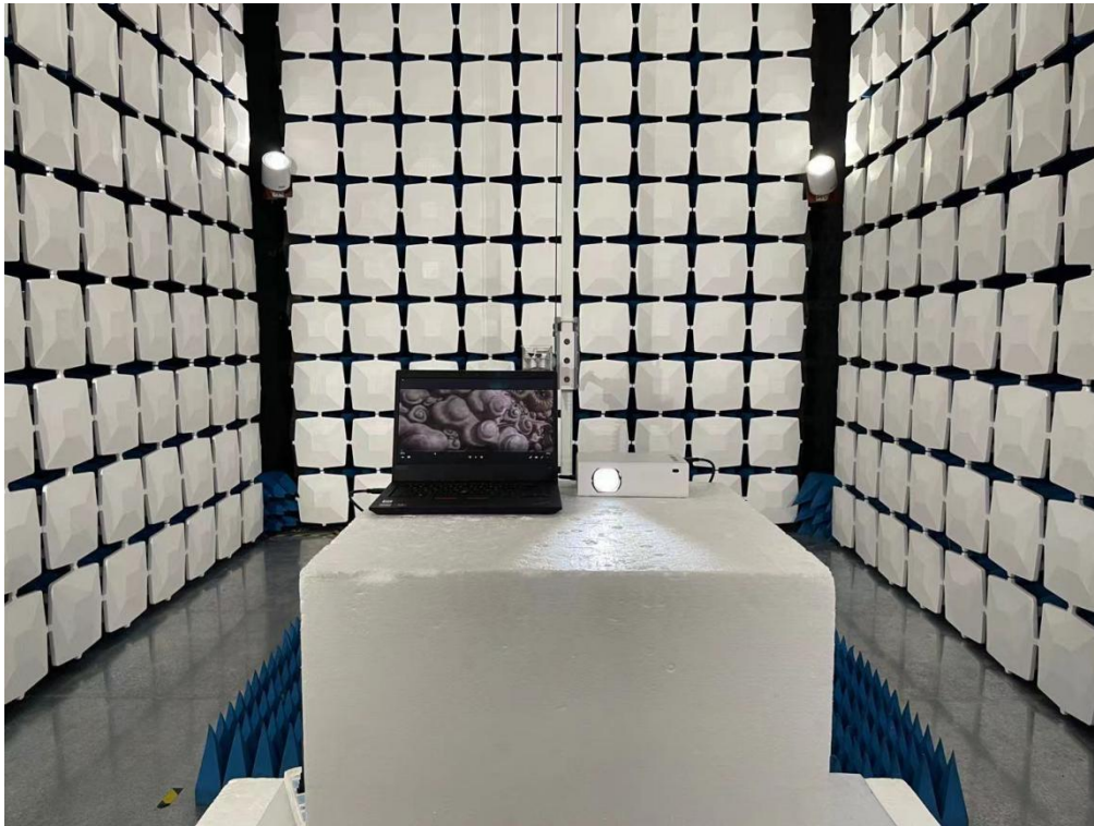
Above 1GHz for radiated emission test setup
