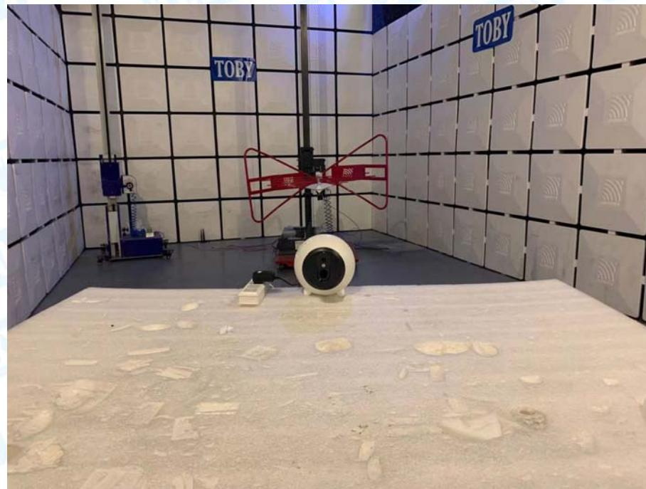
**Photo of Setup for Conducted Emission**
