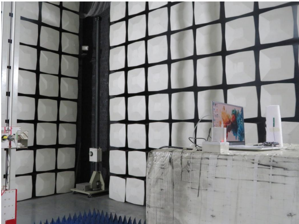
Radiated emission (Above 1GHz) -Antenna RF915-2
