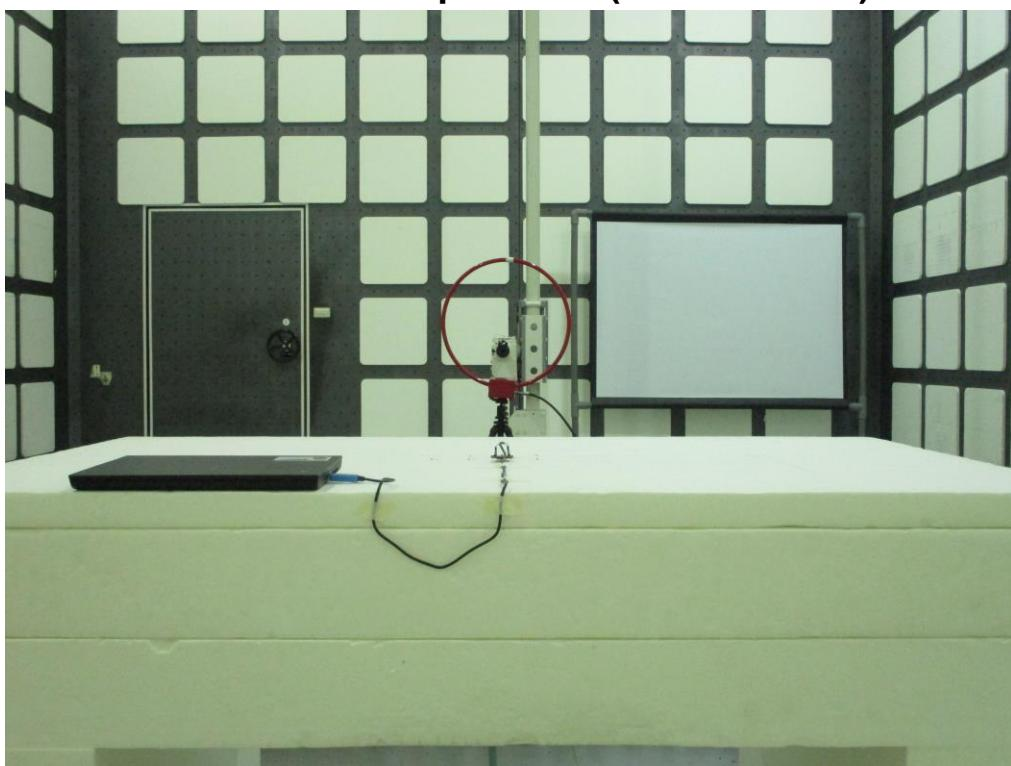
**Radiated Emission Set up Photos (Below 1GHz) BLE 2M**
