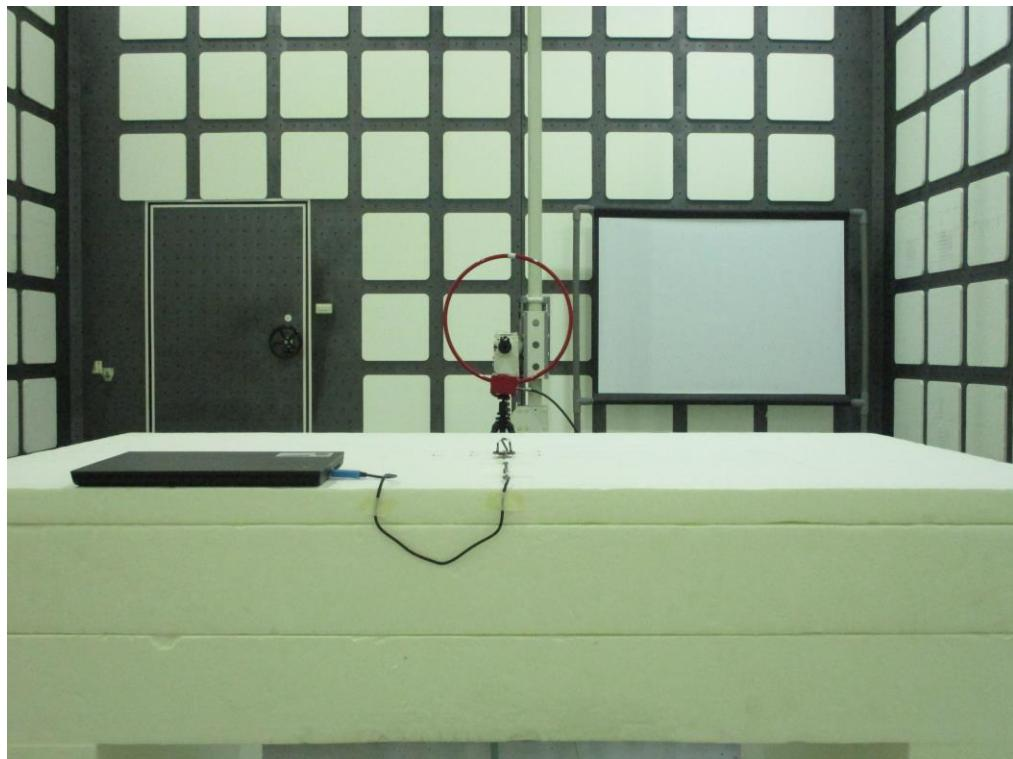
**Radiated Emission Set up Photos (Below 1GHz) BLE 1M**
