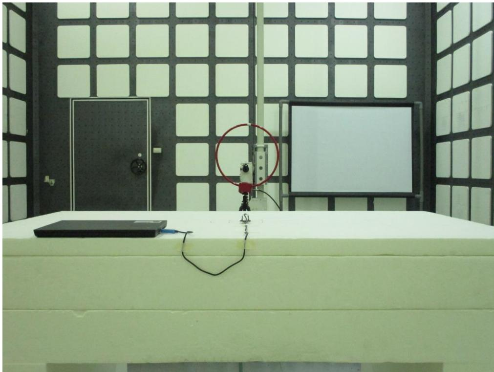
**Radiated Emission Set up Photos (Below 1GHz)**
