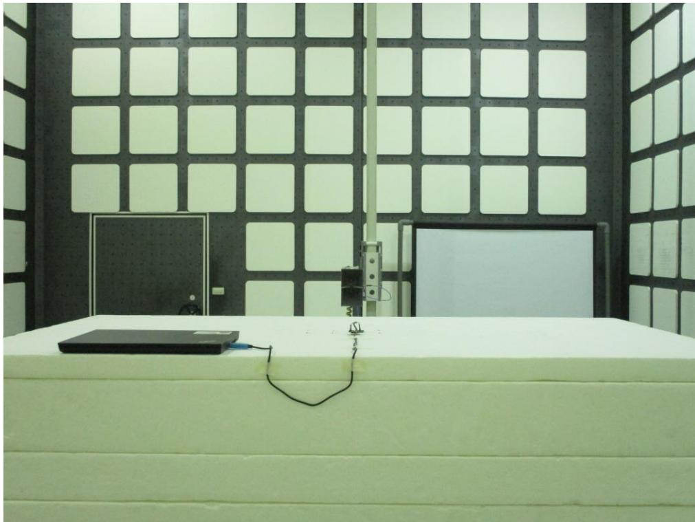
**Radiated Emission Set up Photos (Front View)**
