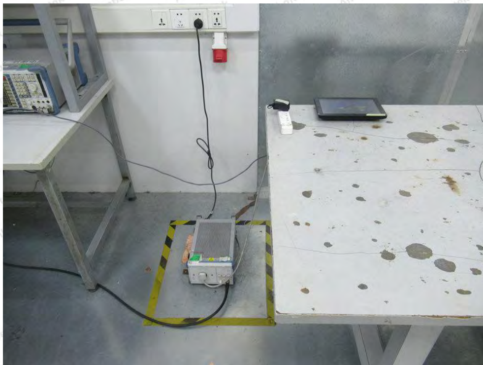
Photo of Conducted Emission Measurement
