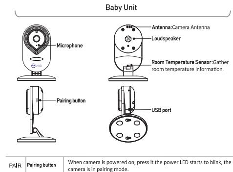
PAIR Pairing button When camera is powered on, press it the power LED starts to blink, the camera is in pairing mode.
