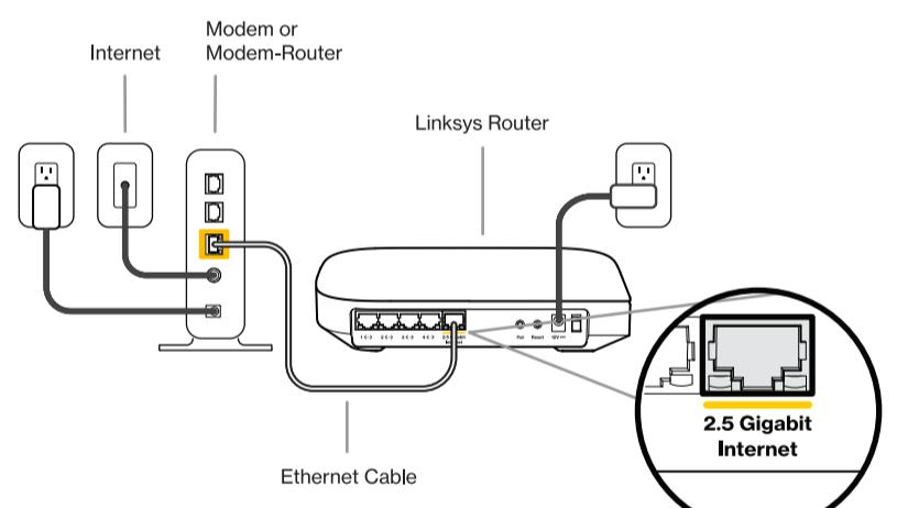
Connect your Linksys Router. Plug it into power, and connect it to your modem with the provided Ethernet cable.
