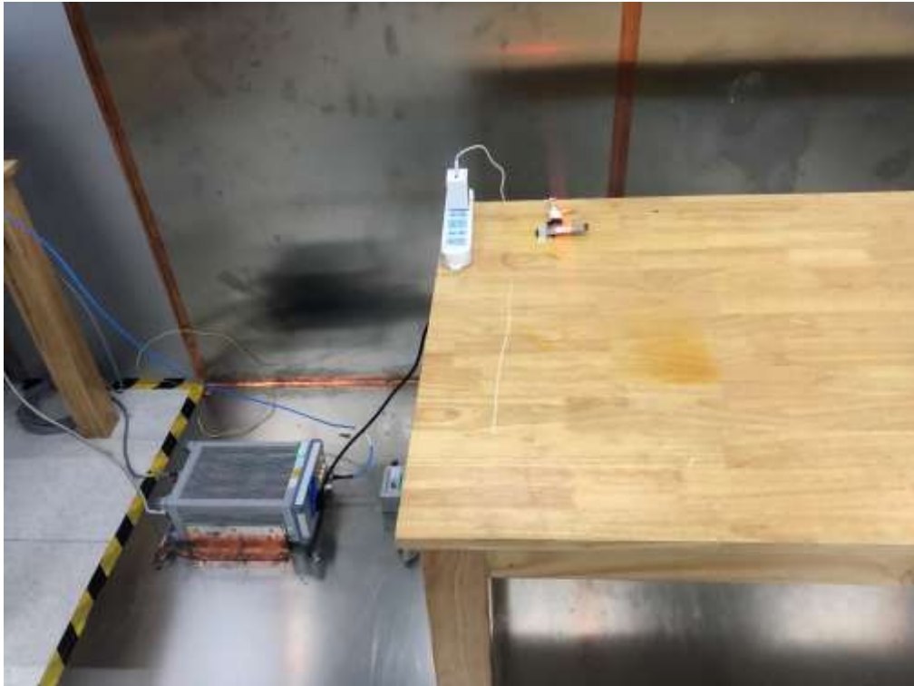
Photograph 3: Set-up photo for Conducted emission
