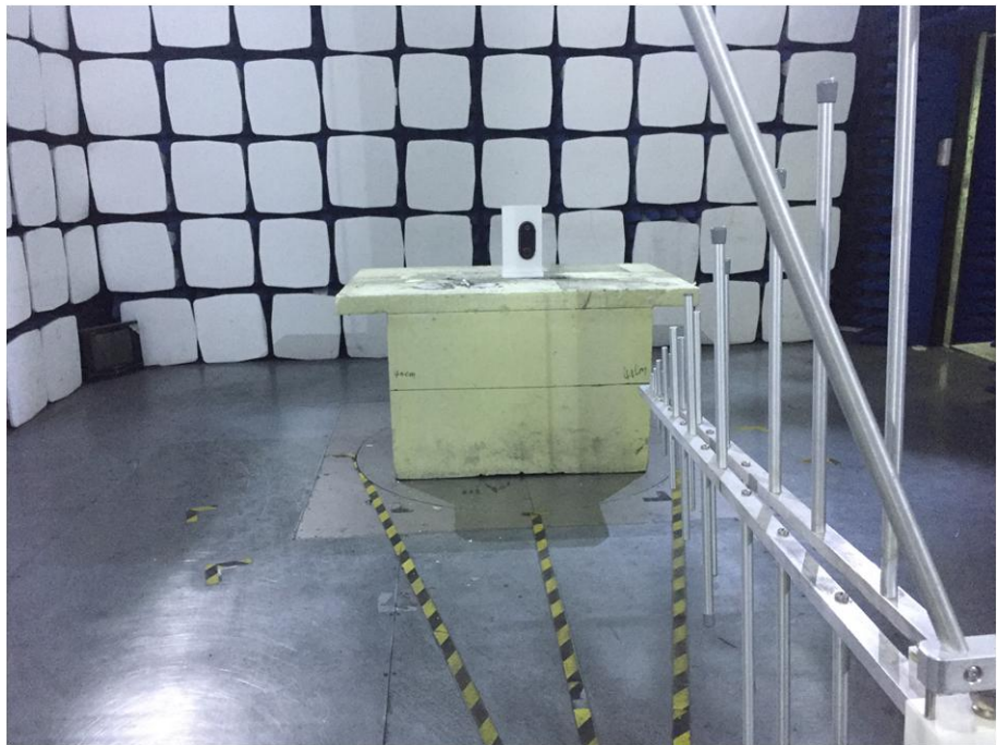
Radiation Emission Test Setup (30MHz to 1GHz)
