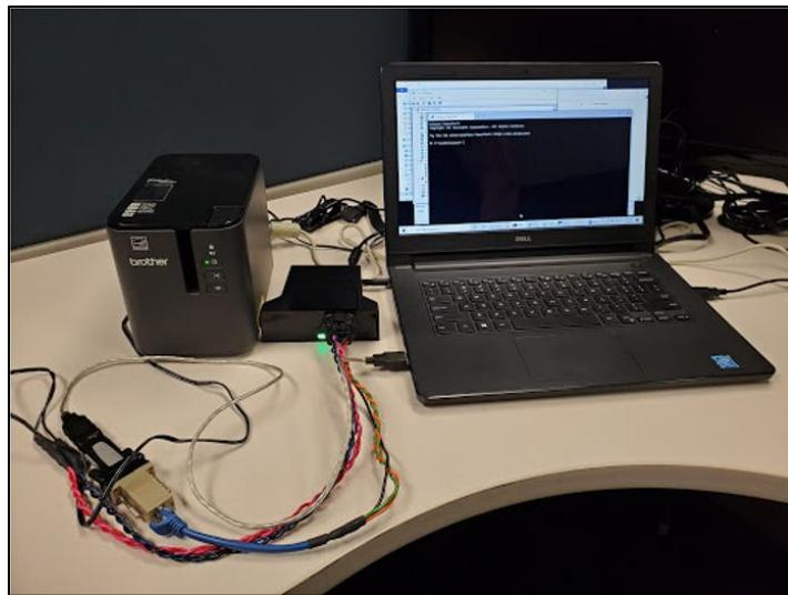
Picture above shows IOTGTWY connected to PC with a diagnostic cable. When connecting to the battery connect the red wire to the red terminal, and the black wire to the black terminal. Plug the USB port into the PC.
