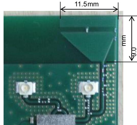
The 50ohm microstrip line and Type2EL\_Antenna needs to be copied when module is installed in the End product.
