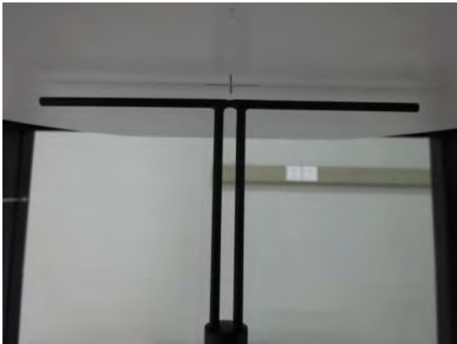
Photo of Dipole Setup
