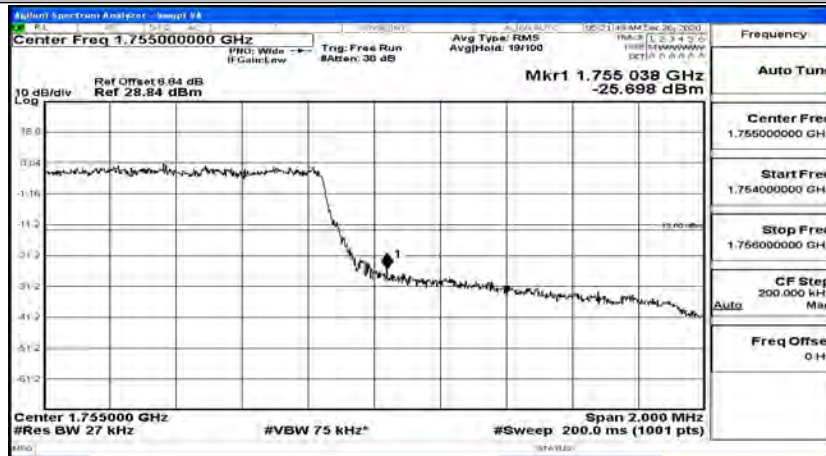
Band Edge Test Graph(s) (Channel Bandwidth: 1.4 MHz)_HCH_16QAM
