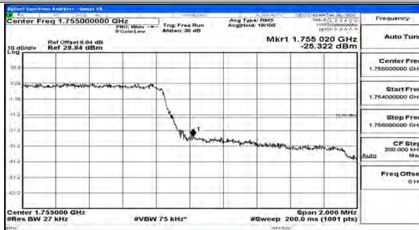
Band Edge Test Graph(s) (Channel Bandwidth: 1.4 MHz)_HCH_QPSK
