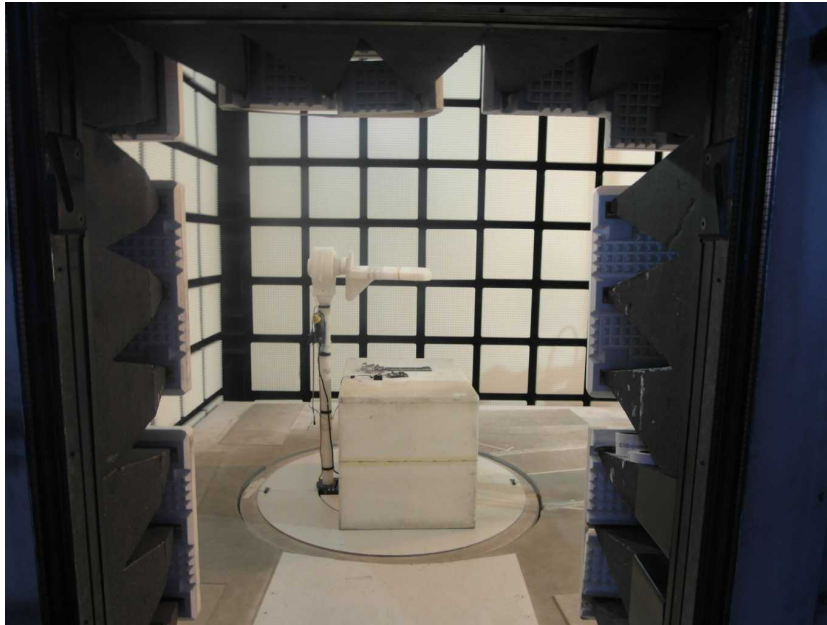
Photo 1: Loop antenna test setup
