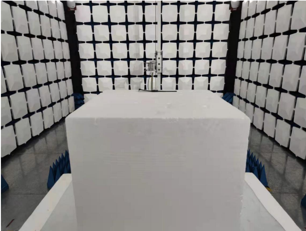
Above 1GHz for radiated emission test setup
