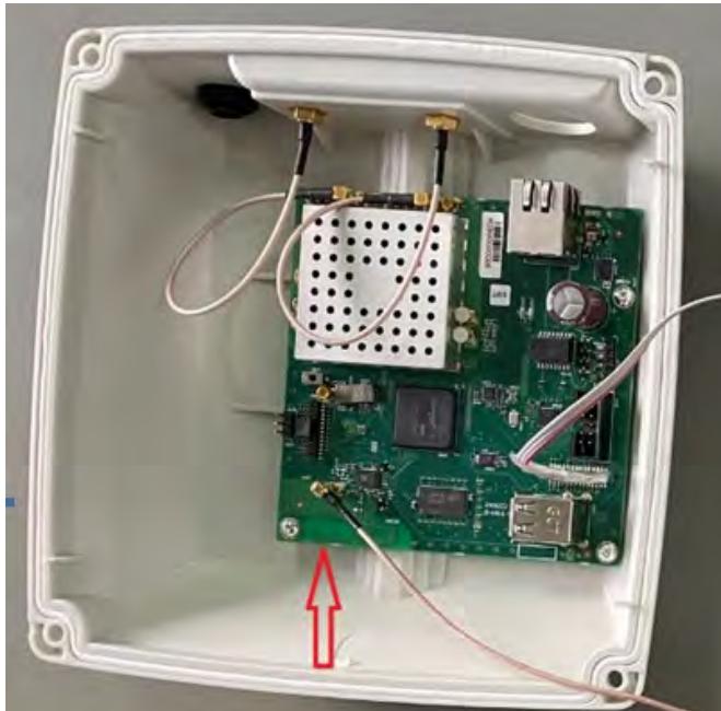
Picture 1 Connection to internal WiFi antenna.
