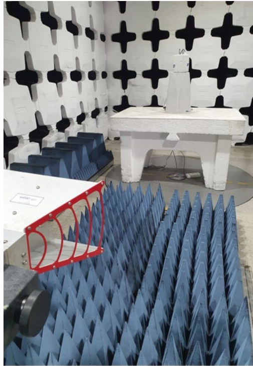
Radiated spurious emission test setup. 1-18GHz
