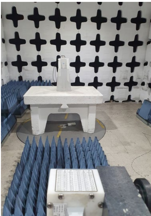
Radiated spurious emission test setup above 18GHz
