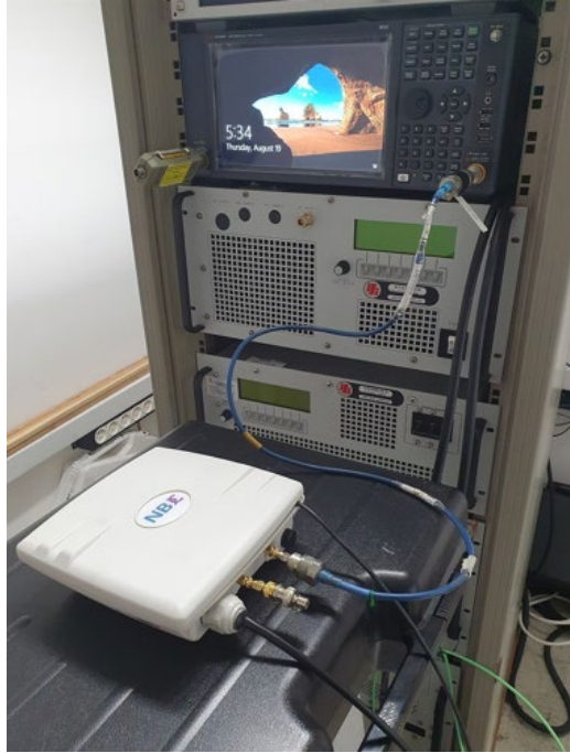
Conducted spurious emission test setup
