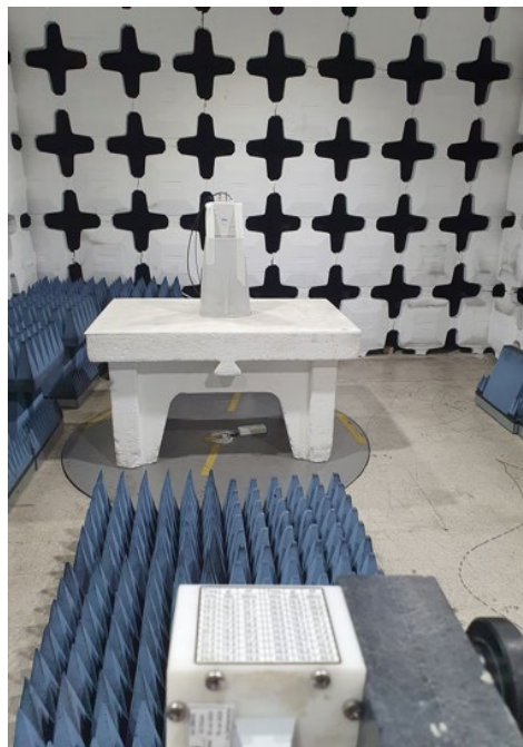
Picture 5 Radiated spurious emission test setup.
