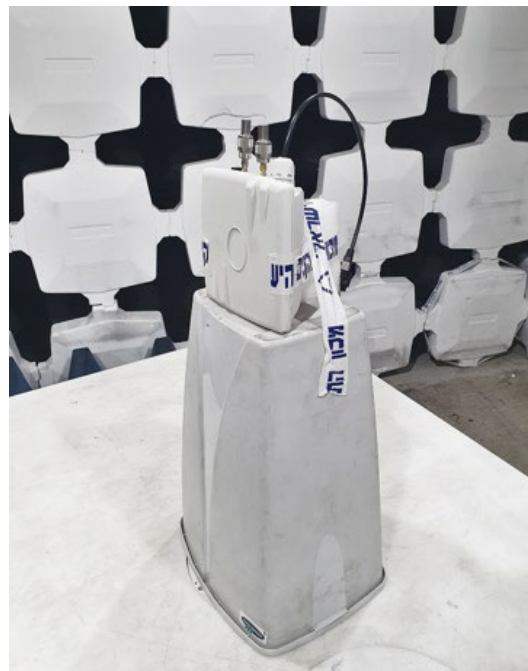
Picture 5 Radiated spurious emission test setup.
