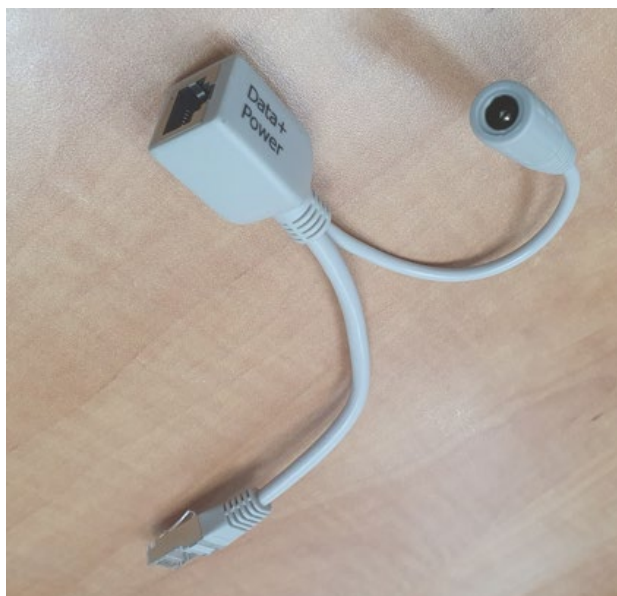
Picture 2. LAN-Power Splitter to use PoE technology
