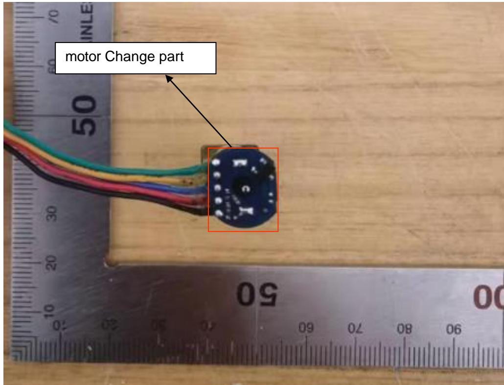
Note: The new model changes the circuit inside the motor to reduce the noise of the product, add reserved structure circuit of U8 for security element and optimize the USB protection design. Main board and wireless RF are same as original model.
