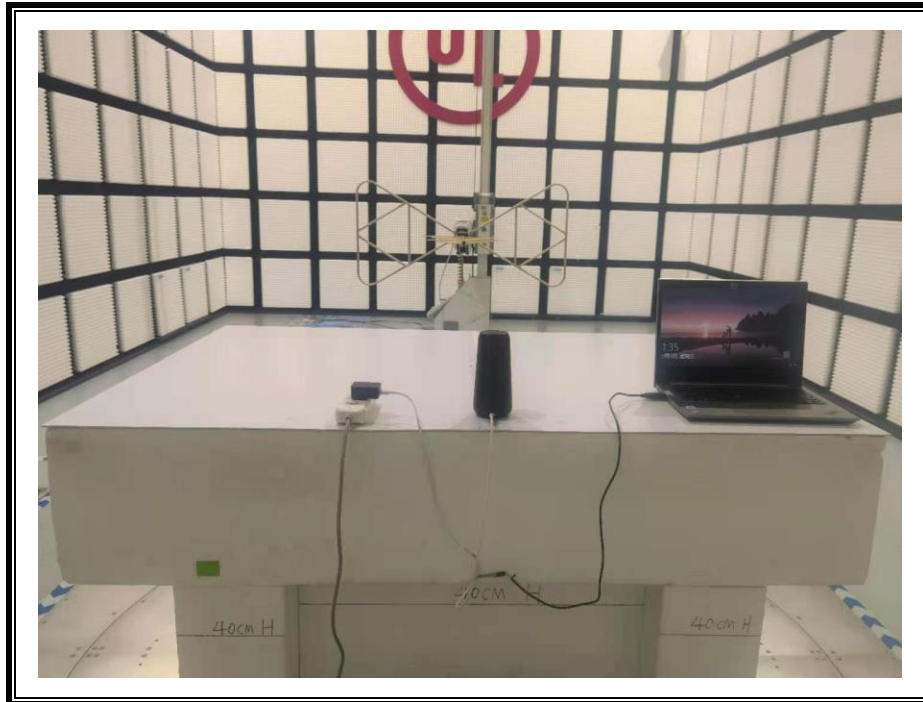
RADIATED RF MEASUREMENT SETUP (Below 30MHz)
