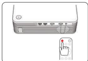
7 Press the power button on the remote control to turn off the projector.
