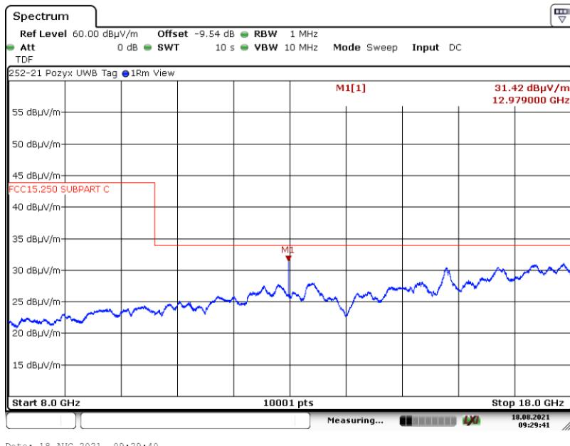
**6.4.36. 8 to 18 GHz Vertical at 1 Meter – Z Axis**
