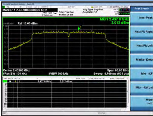
802.11n-40 MHz CHANNEL 5, Carrier level
