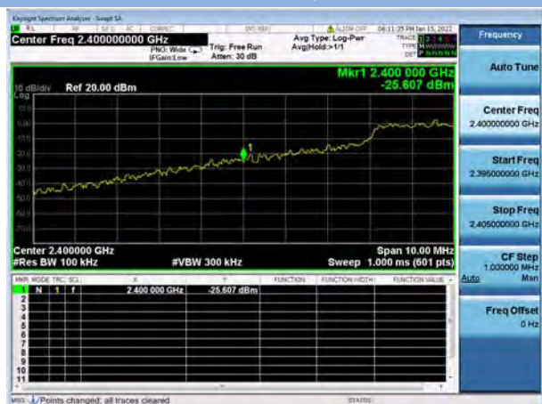
802.11n-20 MHz CHANNEL 1, Reference level
