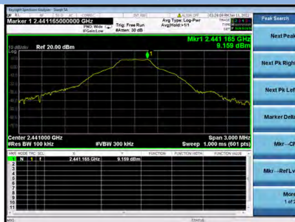
GFSK MIDDLE CHANNEL, CARRIER LEVEL
